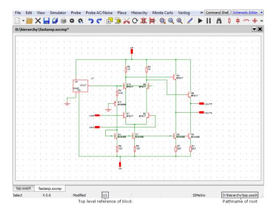
To plot a node in U2, ascend to parent (top.sxsch in the above example) then descend into U2. The same schematic as above will be displayed but will now refer to U2 instead of U1.
