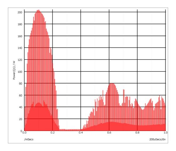
This shows a peak power dissipation of 200W although you are probably more interested in the average power dissipation over a specified time. To display the average power dissipation over the analysis period:
