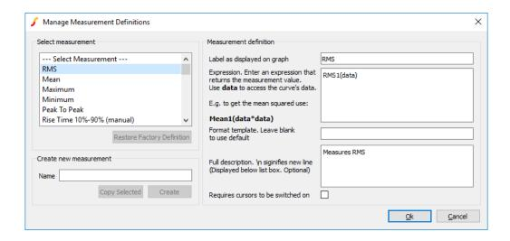
The Measurement Definitions Manager allows you to edit both built in and custom measurement definitions.
