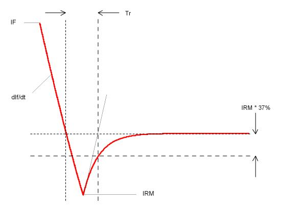
The reverse recovery characteristics are explained in the following diagram.
