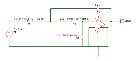
The above circuit is that of a two pole low-pass filter. C1 is fixed and R1=R2. The design equations are:
