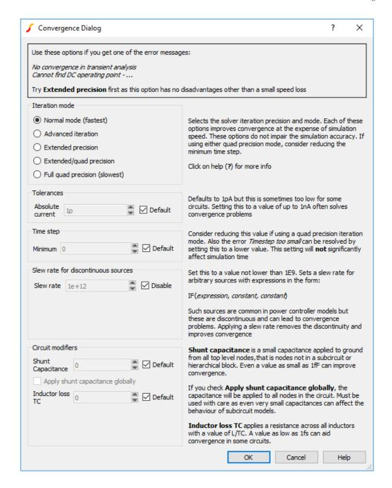
This dialog allows to set a number of simulation options that can help simulation convergence. These options sometimes have a penalty, either they slow down the simulation or in some way degrade accuracy. These are described below
