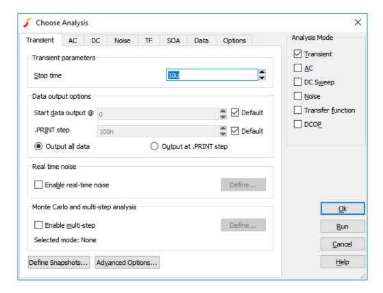
Click AC check box and uncheck the Transient check box. The details of the AC sweep have already been set up - click the AC tab at the top to see them.
