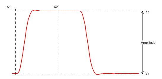
Function returns the 10% to 90% rise time of the first rising edge that occurs between x1 and x2. The 10% point is at y threshold Y1 + (Y2-Y1)\*0.1 and the 90% point is at y threshold Y1 + (Y2-Y1)\*0.9.
