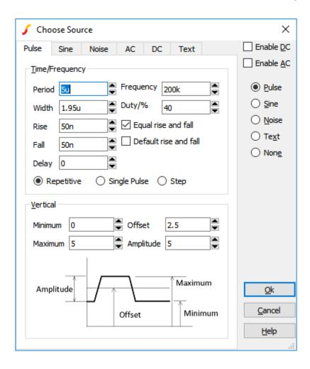
This sets up a 200kHz 5V pulse source with 40% duty cycle and 50nS rise time.
