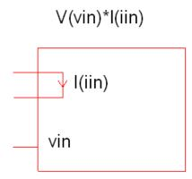
The result plotted will be the product of the voltage on vin and the current in iin.
