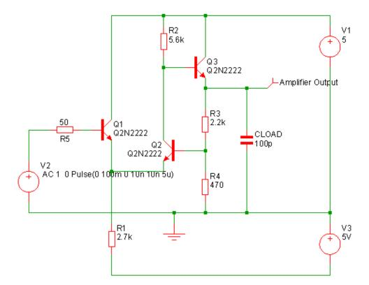
This is a simple feedback amplifier designed to amplify a 100mV pulse up to around 500mV. The
