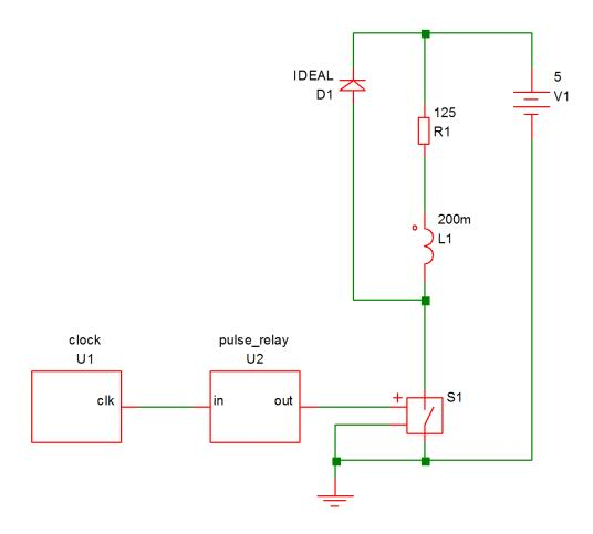
This circuit pulses a relay for 10mS every 100mS driven by a 100kHz clock. The relay coil is modelled by L1 and R1 while D1 is a freewheel diode. S1 is the relay driver and is controlled by the output of U2. This is a simple counter implemented using the following Verilog code:
