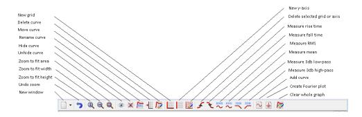
The above shows the function of each of the buttons on the graph toolbar. These are referred to in the following sections.
