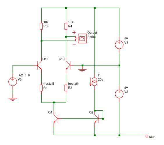
The following is the result of a DC sweep of V3 with restail set to 1K. Analysis parameters were as follows:
