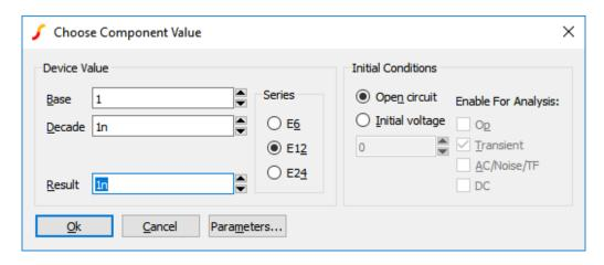
You can type the new value in directly in the Result box or you can select a value using the mouse alone with the up and down arrow buttons. Leave the Initial Conditions setting at its default (Open Circuit)
