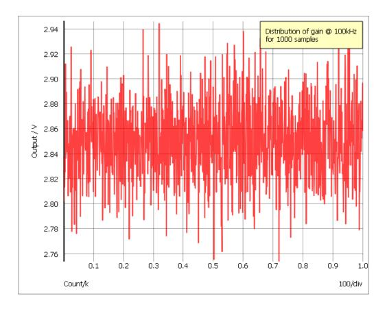
The graph shows the variation in gain for 1000 samples. Using the histogram feature a statistical distribution of the above can easily be plotted.
