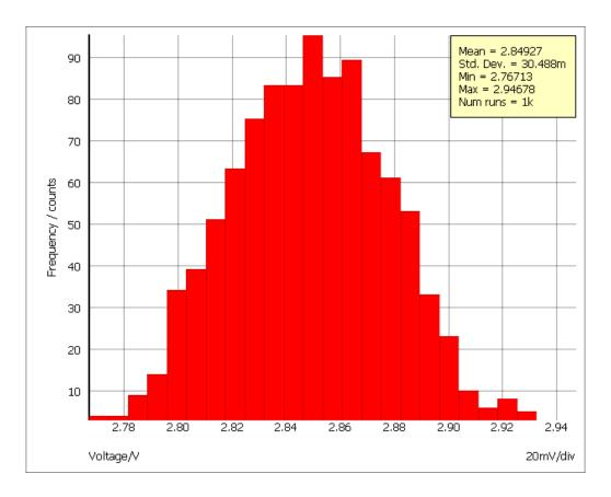
This is a histogram showing the distribution of the gain of the amplifier at 100kHz.
