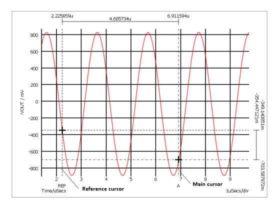
The cursors can be moved horizontally or vertically while tracking an attached curve or they can be picked up and dragged onto another curve.
