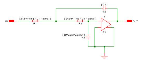
You can set the values of the parameters for each instance of the above subcircuit by appending the expressions to the VALUE property of the symbol in the main circuit separated by a ':'. E.g.:-
