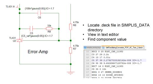
In the above diagram, note the line for C5 shows a value of 2.2797033192142e-008 in the .deck file
