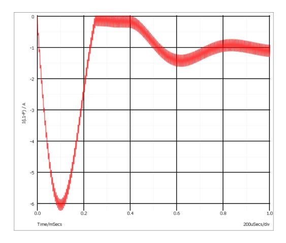
This shows that the operating current is less than 1.5A but peaks at over 6A. In practice you would want to use an inductor with a maximum current of around 2A in this application; an inductor with a 6A rating would not be cost-effective. We will now replace the ideal part, with something closer to a real inductor.
