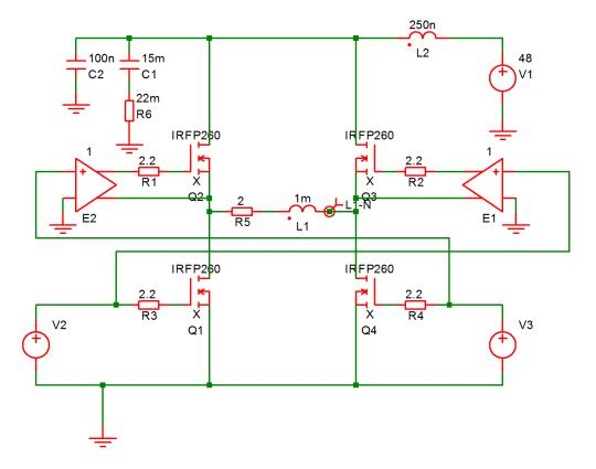
Sources V2 and V3 have been defined to be dependent on a parameter named *duty* which specifies the duty cycle of the switching waveform. See EXAMPLES/BRIDGE.sxsch.
