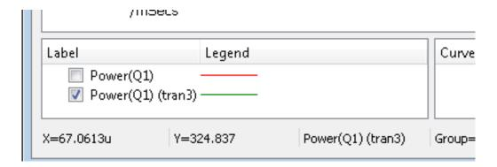
6. As before, press **F3** then select Mean with the cursor span pre-process option. The new peak power cycle will now be in the 11-12W region - much more than before.
