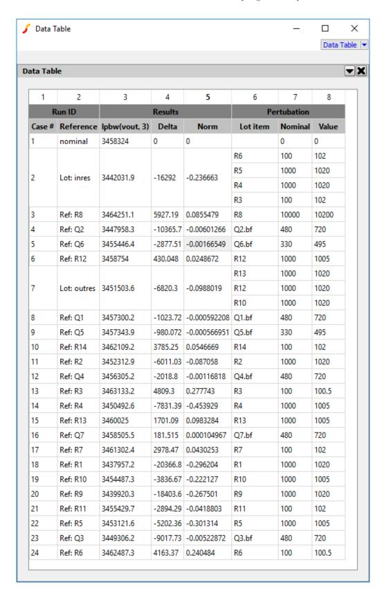
Double-clicking the headings will sort the values in order of magnitude or alphabetically in the case of the Reference column. Sorting is inactive for the Perturbation columns.
