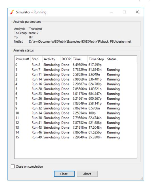
The above shows the status box showing for a 1000 step Monte Carlo analysis using 8 cores. Each line shows the status for each of the 8 processes. Apart from sending back status information, each of the 8 processes runs completely independently and writes to its own data file. When the run is complete the data from each processes will be linked to the main data file. Subsequently you can plot and analyse the results in exactly the same way as you would a single core run.
