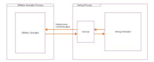
vsxd.vpi is a DLL/shared library that is provided as part of SIMetrix. This is loaded by the external Verilog simulator and runs in the Verilog process's memory space. vsxd.vpi uses the VPI interface to send events to the Verilog simulator, to respond to events generated by the Verilog simulator and to interrogate the Verilog simulator about details of the user's Verilog module.
