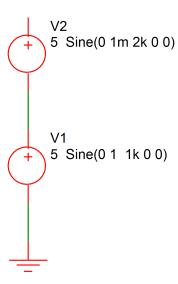
The signal on the pos side of V2 has 0.1% distortion. Use V1 as your main test source (assuming you are testing an amplifier) then after the simulation is complete, check that the distortion measurement of V2 is 0.1%. If it is inaccurate, you will need either to increase the number of measurement cycles or reduce the maximum time step or both. You can adjust the amplitude of V2 appropriately if the required resolution is greater or less than 0.1%.
