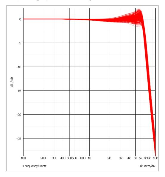
As can be seen, the specification is generally met. In the next section "Sensitivity/Worst-case Example" on page 415 we will perform a worst-case analysis on the circuit which will show that there are extreme combinations of values that do not meet the spec.
