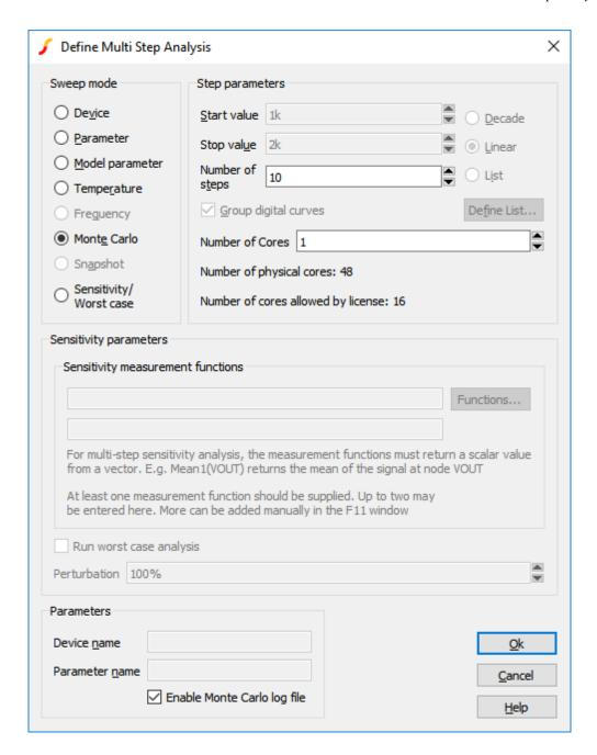
Enter parameter as described below. Only the boxes for which entries are required will be enabled. In the above example, only the Number of steps box is enabled as this is all that is required for Monte Carlo mode.
