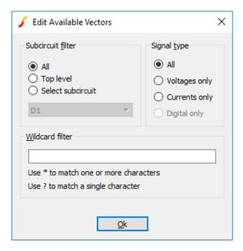
This allows you to select what is displayed in the available vectors dialog. This is useful when simulating large circuits and the number of vectors is very large.
