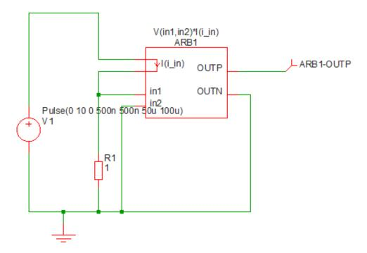
In the above, ARB1 is the device created from the Non-linear Transfer Function menu. ARB1-OUTP will carry a voltage equal to the power dissipation in R1.
