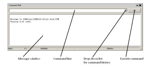
The command line is at the top of the command shell. See diagram above.
