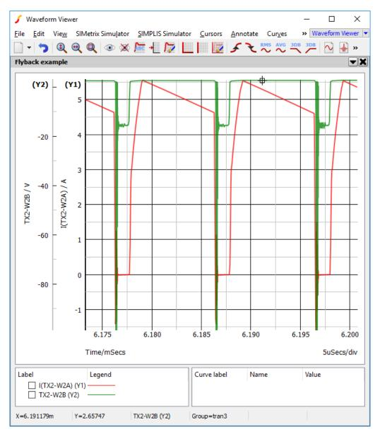
Current and Voltage plotted on separate Axes
