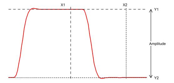
Function returns the 10% to 90% fall time of the first falling edge that occurs between x1 and x2. The 10% point is at y threshold Y1 + (Y2-Y1)\*0.1 and the 90% point is at y threshold Y1 + (Y2-Y1)\*0.9.
