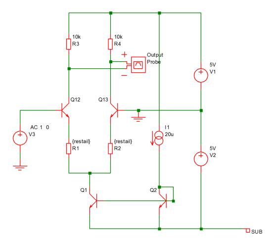
This is a simple long tailed pair. The above circuit resistors R1 and R2 have been given the values {restail}. *restail* is a parameter that is swept in an AC sweep to plot the gain of the amplifier vs tail resistance at 100kHz. Here is the result of the run:
