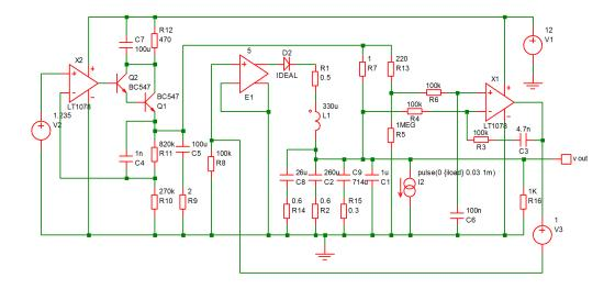
I2 provides a current that is switched on for 1mS after a short delay. A multi-step analysis is set up so that the load current is varied from 10mA to 1A. The output for all runs is:
