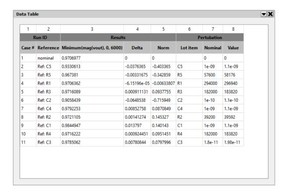
The Delta column shows the deviation from the nominal for each case. Double-click the Delta label in the header. This will sort the results in order of magnitude and so show which cases had the greatest effect. Note that C2 and C5 are at the top of the list. We will now tighten the tolerance on these parts to 2%. To do this:
