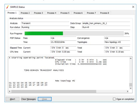
You can watch the progress of each process using the tabs at the top of the status box.
