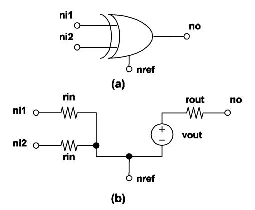
4.10 Exclusive-OR gate model: (a) Symbol for exclusive-OR gate, (b) Model for exclusive-OR gate. The nodes ni1 and ni2 are the two input nodes. The nodes no and nref are the output and reference nodes, respectively.
