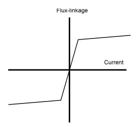
9.17b Flux-linkage vs. current characteristics of inductor
