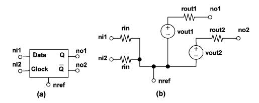
4.15 Clocked Data Flip Flop model: (a) Symbol for a SIMPLIS Clocked Data flip flop, (b) Model for a SIMPLIS Clocked Data flip flop.
