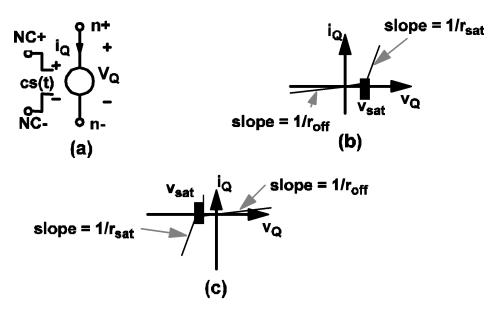
4.4 Model for the simple transistor switch: (a) Simple transistor switch controlled by a control signal cs(t), (b) the i Q vs v Q characteristic of the simple POS-type transistor switch, and (c) the i Q vs v Q characteristic of the simple NEG-type transistor switch.
