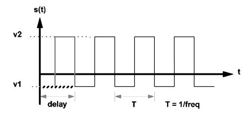
3.4 Waveform s(t) of a square wave source
