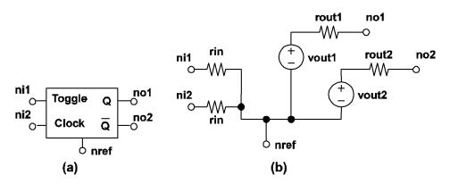
4.16 Clocked Toggle Flip Flop model: (a) Symbol for a SIMPLIS Clocked Toggle flip flop, (b) Model for a SIMPLIS Clocked Toggle flip flop.
