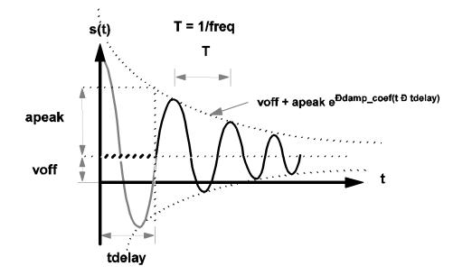
3.6 Waveform s(t) of a sinusoidal source
