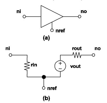
4.8 SIMPLIS inverter model: (a) Symbol for inverter, (b) Model for inverter. The nodes ni, no and nref are the input, output and the reference nodes, respectively.
