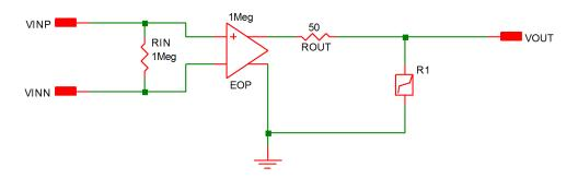
9.7b Example 3 Operational Amplifier with Saturation - Piecewise-linear Equivalent Circuit
