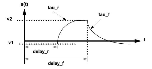
3.8 Waveform s(t) of an exponential pulse source
