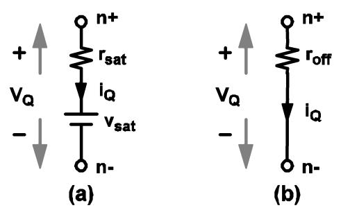
4.5 Model for the simple transistor switch: (a) model of the simple transistor switch for LEVEL=1 when it is in a closed state, and (b) model of the simple transistor switch for LEVEL=1 when it is in an open state.
