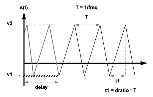
3.3 Waveform s(t) of a triangular source
