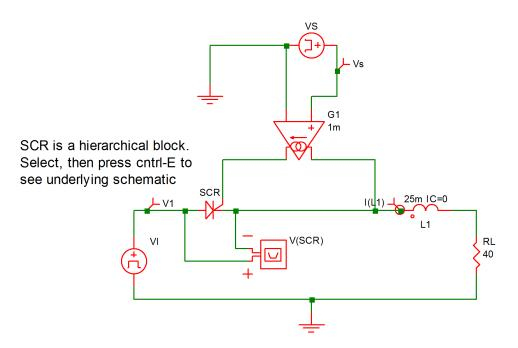
9.20 Example 7: A silicon-controlled rectifier with series R-L load.
