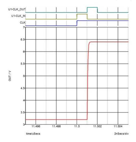
A discrete filter with more than two poles can be synthesized through a cascade of one-pole and/or two-pole discrete filters. In such case, the timing signal for each driven stage is derived from the "CLK\_OUT" signal of the immediately preceding stage.
