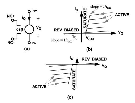
4.6 Model for the simple transistor switch for LEVEL=2. (a) A simple transistor switch controlled by a control signal cs(t), (b) The i Q vs v Q characteristics of a VCQPOS-type or ICQPOS-type transistor switch, (c) The i Q vs v Q characteristic of a VCQNEG-type or ICQNEG-type transistor switch.
