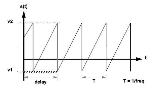
3.2 Waveform s(t) of a sawtooth source
