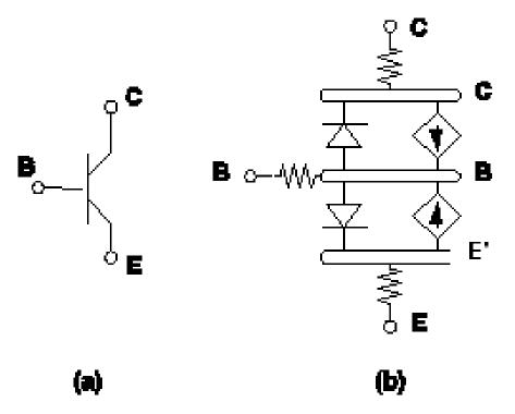
5.1 Ebers-Moll model of an NPN transistor: (a) Circuit symbol, (b) the Ebers-Moll model. Note: B', C', and E' are the internal nodes introduced for modelling purposes.
