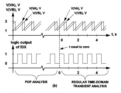
10.5 (a) Waveforms of two periodic sawtooth voltage sources VA and VB when no periodic operating point analysis is carried out, and (b) Waveform of the same voltage source when a periodic operating point analysis is carried out. The start of a switching cycle is defined as occurring when the output of the logic gate !DX is making a 0 to 1 transition.
