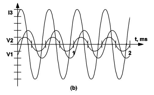
11.1 Waveforms for the small-signal AC source examples V1, V2, and I3.
