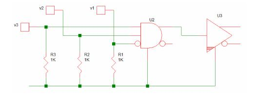
In this example, you should assign zero delay to U2, the classic 3-input AND gate and the non-zero delay to U3, the Advanced Digital buffer.
