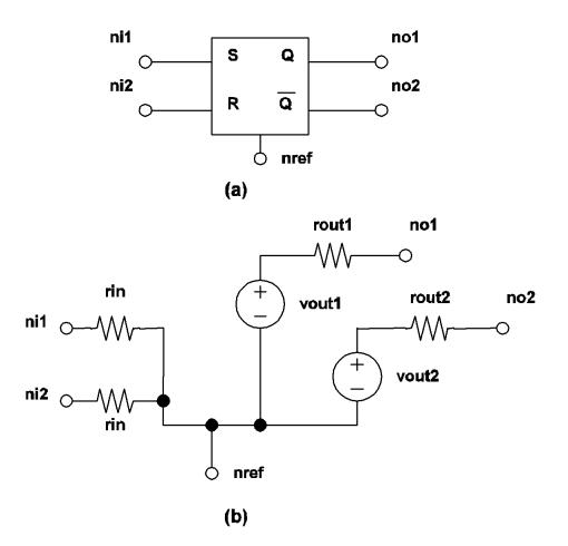
$4.12~{\rm SR}$  Flip Flop model: (a) Symbol for a SIMPLIS S-R flip flop, (b) Model for a SIMPLIS S-R flip flop.
