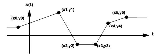
3.9 Example of the waveform  $\mathbf{s}(\mathbf{t})$  of a typical piecewise-linear source
