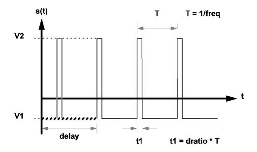
3.5 Waveform s(t) of a pulse-wave source
