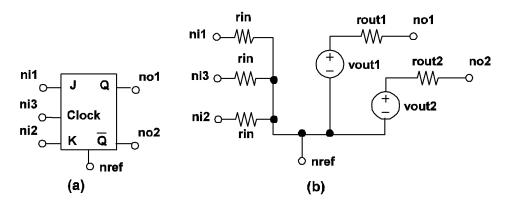
4.14 Clocked J-K Flip Flop model: (a) Symbol for a SIMPLIS Clocked J-K flip flop, (b) Model for a SIMPLIS Clocked J-K flip flop.
