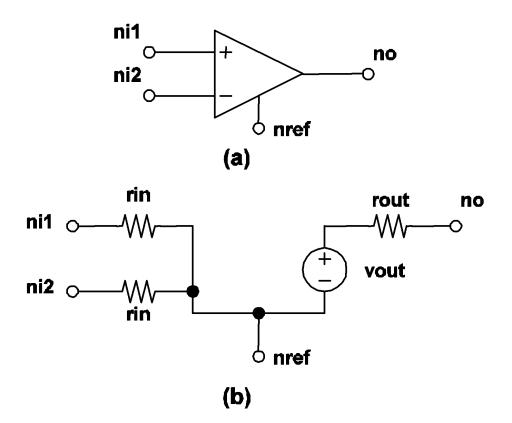
4.9 SIMPLIS comparator model: (a) Symbol for comparator, (b) Model for comparator. The nodes n1, n2 are the two input nodes. The nodes no and nref are the output and reference nodes, respectively.
